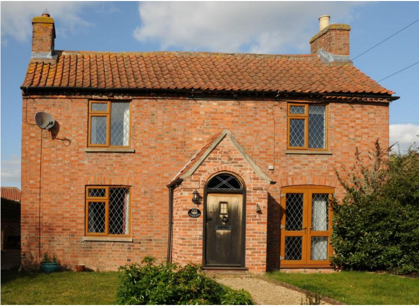
1: A typical late C19 brick and pantile cottage with chimneys creating a symmetrical elevation albeit with a recent porch. Brick coursing shows contrasting headers and stretchers.
